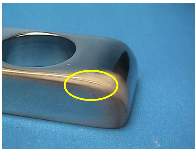
Figure 1. Chrome burn on a 334 cylinder control housing
