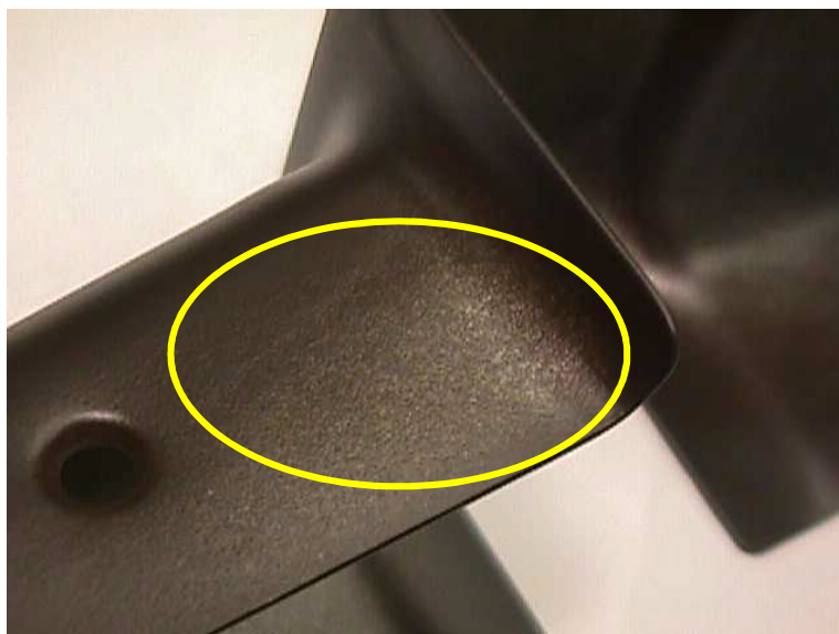
Figure 6. Light Paint Coverage on a One Piece Center Case Cover.
